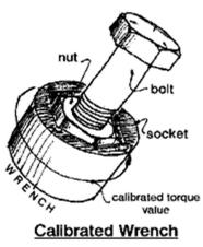
As with every bolt pretensioning method, Calibrated Wrench may only be performed after all steel plies in a connection have been drawn into firm contact, i.e. snug-tightened. Failure to do so will result in inadequate bolt pretension and loose connections.
