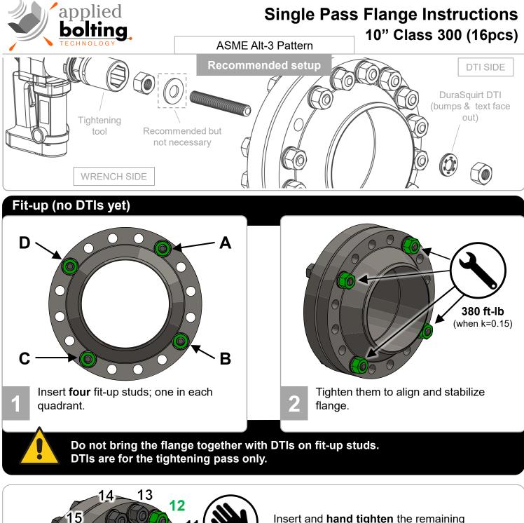
Insert and **hand tighten** the remaining hardware, now including DTIs.
