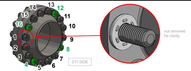
Confirm the DuraSquirt DTIs were installed correctly and the fit-up ones are available, which will get installed in step 6.
