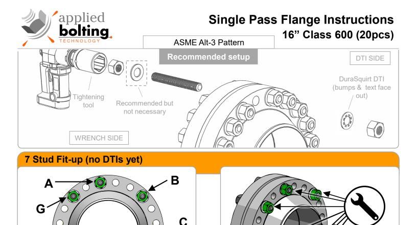
Begin by inserting one stud, skip the next two holes, insert the next stud... Repeat this pattern around the flange as shown.
