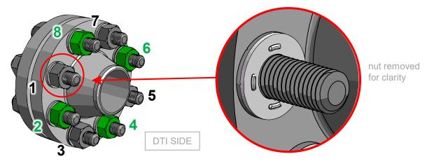
Confirm the DuraSquirt DTIs were installed correctly and the fit-up ones are available, which will get installed in step 6.
