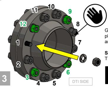
Insert and **hand tighten** the remaining hardware, now including DTIs.
