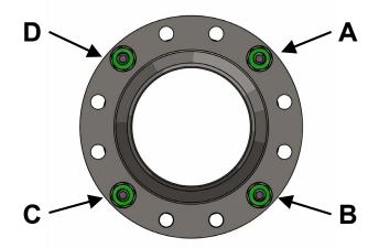
Insert **four** fit-up studs; one in each quadrant.
