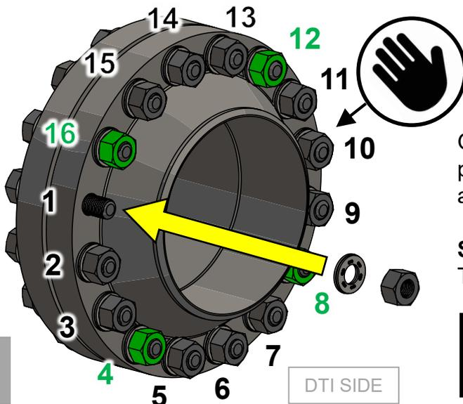
Insert and **hand tighten** the remaining hardware, now including DTIs.
