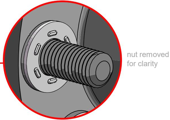
**4** Confirm the DuraSquirt DTIs were installed correctly and the fit-up ones are available, which will get installed in step 6.
