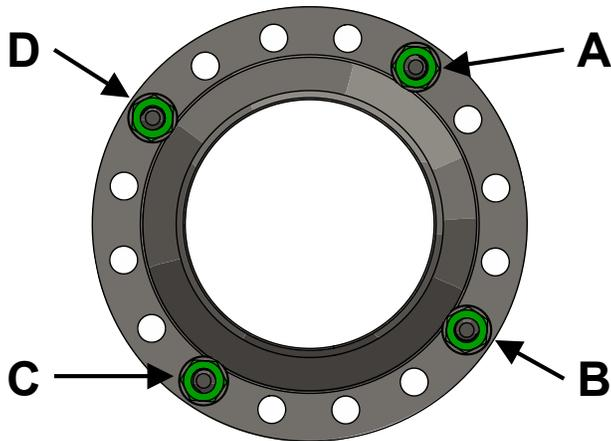
**1** Insert **four** fit-up studs; one in each quadrant.
