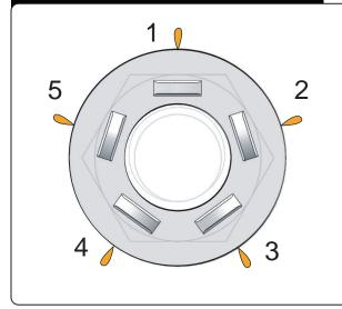
When orange is visible from all bumps, installation and inspection is complete.
